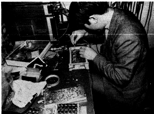
JA1CBL of Japan AMSAT Association (JAMSAT) building parts of the Mode J transponder.
