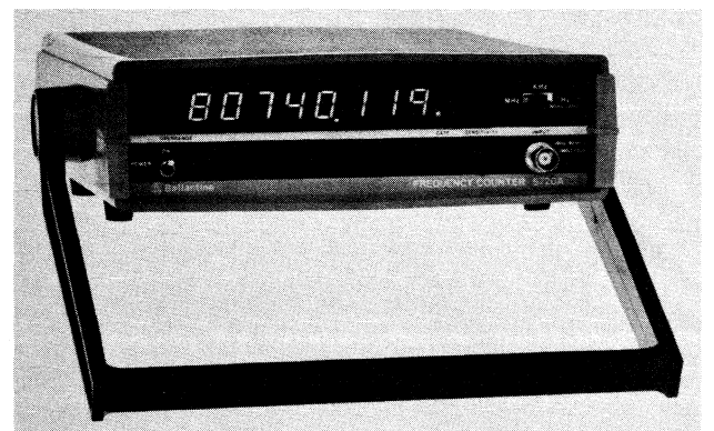
Ballantine's model 5720A Frequency Counter covers the range from 10 Hz to more than 80 MHz and provides frequency and ratio measurements. This counter also includes an audio multiplier circuit for input frequencies from 50 Hz to 1 kHz which provides resolution of 0.01 Hz with only 1-second measurement time ( photo courtesy Ballantine Laboratories).
