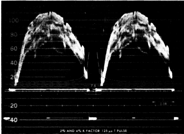
fig. 3. Horizontal video waveform as seen on an analyzer. The sync pulse is seen on the -40 line.
