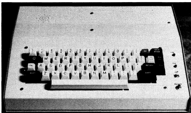
The CW keyboard is housed in a 14 x 11 x 3 inch (36x28x8 cm) cabinet available from Nu Data Electronics, 104 North Emerson Street, Mount Prospect, Illinois 60056.
