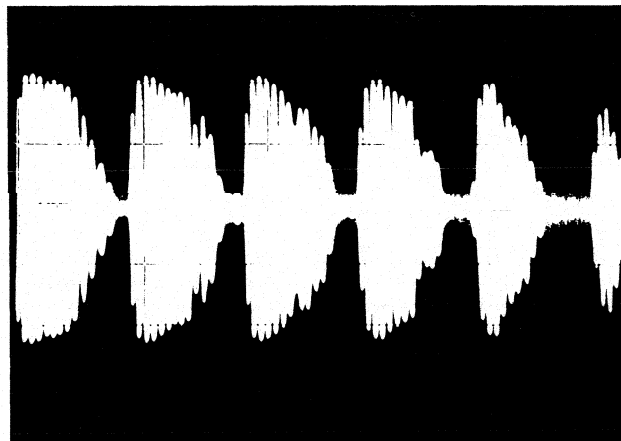
Transverter output on 80 meters showing ssb (upper) and CW (lower) modes as viewed on a Hewlett-Packard model 182 oscilloscope.
